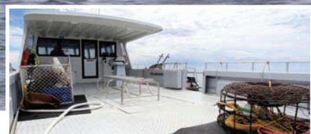
The 'Aqua Jade' has a sizable aft working deck, complete with a Cloverdale Pumps pot hauler and access to the 300kg live lobster storage hold
